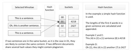
Figure 4: Concept of Fingerprinting
