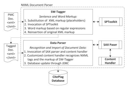
Figure 22: Two-stage Parsing Process for NXML Documents
