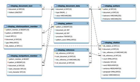
Figure 23: ER Data Model for the CitePlag Database
