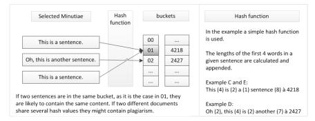
Figure 4: Concept of Fingerprinting
