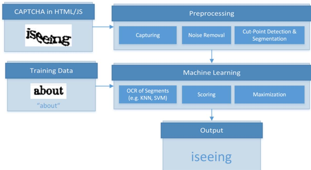
Figure 2: Generic process for solving static text CAPTCHAs
